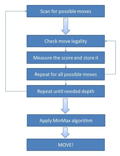
Figure 1: Chess program overall structure (simple version)
